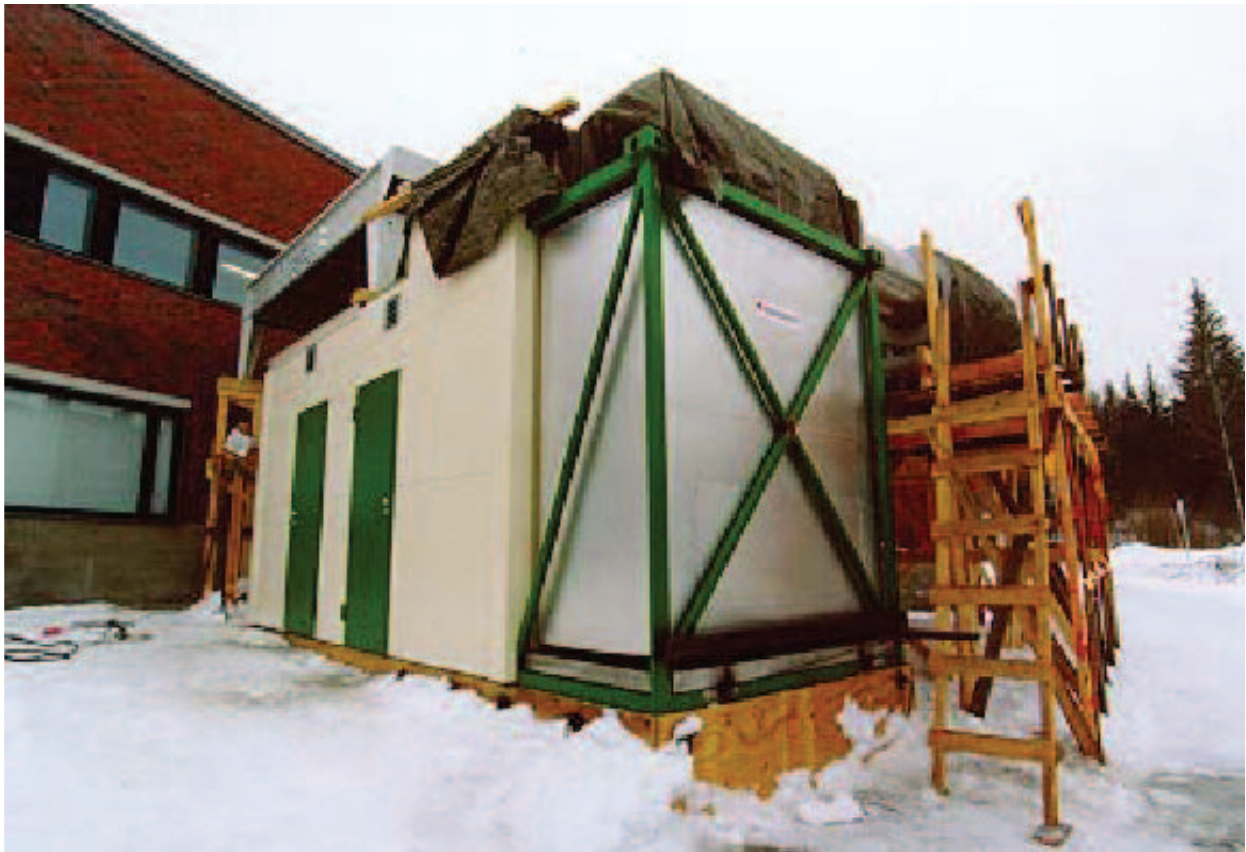
Fig 3 High speed ORC power plant container on the test site
