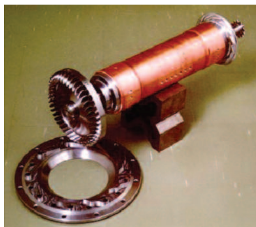
Fig 5 Stator nozzle ring (one half), turbine rotor, generator rotor, cooling fan, pump impeller
